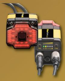
The FlexVision controller is an integrated device that provides all logic and connectors to connect cameras, encoders and an alarm plus handle digital inputs and digital outputs.
